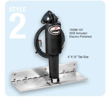
Blades are constructed of 12 gauge (2.7 mm) laser cut 304 stainless steel with a folded over trailing edge for safety, welded on lower mounting brackets & 1/8" (3.2 mm) diameter hinge pin. High impact corrosion proof upper mounting brackets with mechanical cable gland seal.
