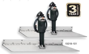
Blades are constructed of 7 gauge (4.6 mm) laser cut 304 stainless steel with 3/8 (9.5 mm) diameter hinge pin. High impact corrosion proof upper mounting brackets with mechanical gland cable seal and stainless steel welded on lower brackets, 5/16" (.8 cm) upper and 3/8" (9.5 mm) lower stainless steel mounting bolts. 3.75" (9.5 cm) sacrificial anodes installed.
