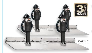
Blades are constructed of 7 gauge (4.6 mm) laser cut 304 stainless steel with 3/8 (9.5 mm) diameter hinge pin. High impact corrosion proof upper mounting brackets with mechanical gland cable seal and stainless steel welded on lower brackets, 5/16" (.8 cm) upper and 3/8" (9.5 mm) lower stainless steel mounting bolts. 3.75" (9.5 cm) sacrificial anodes installed.
