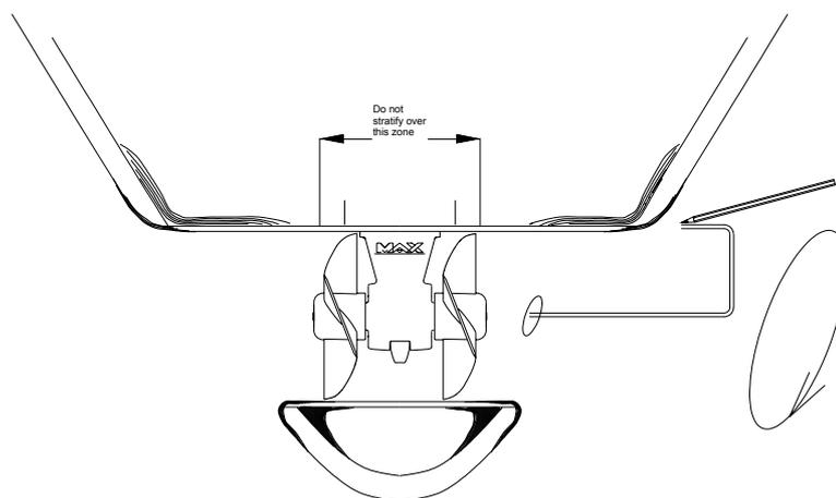
Fit the tunnel and mark the areas to be fibre-glassed. Sand these areas inside and out.
