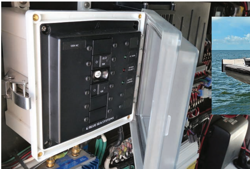
Metal Shark boats builds custom aluminum boats for government agencies and relies on the Blue Sea Systems Surface Mount System (SMS) box with ELCI aboard the Relentless 28.
